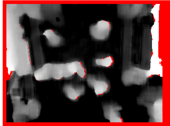
(a) The depth image by the stereo camera. Red regions represent pixels for which no stereo value could be computed.
