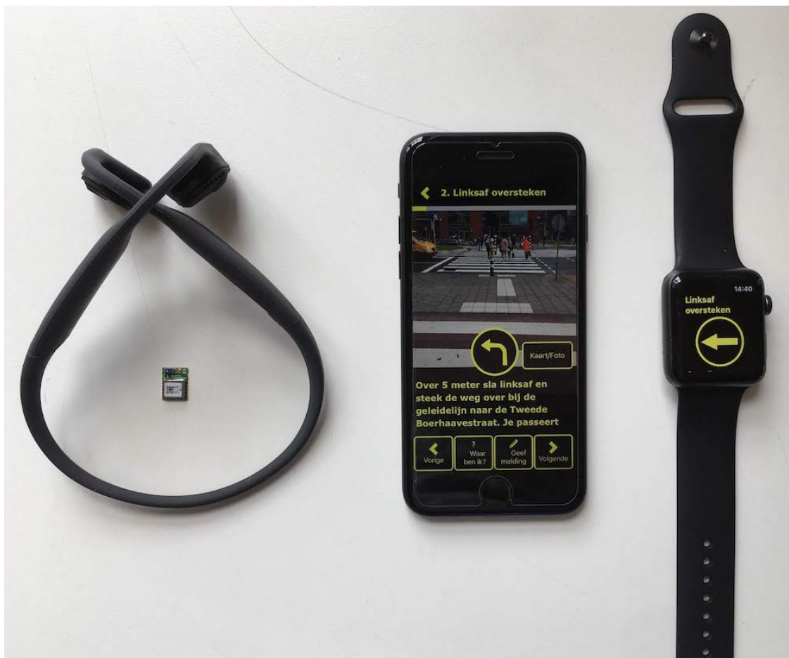
Figure 3: Bone conducting headset, iPhone and Apple watch app prototype for wayfinding via multi-modal communication. A message used in session 7 and 8 is displayed on the devices.
