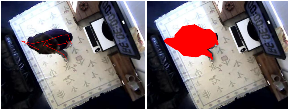
Figure 8: The skeleton reprojected into the overhead camera image. Next to it is the expanded skeleton reprojected into the same camera image.
