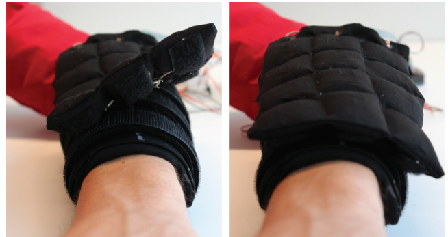
Figure 1: The TaSST. The input layer is attached to the top of the output layer using Velcro.
