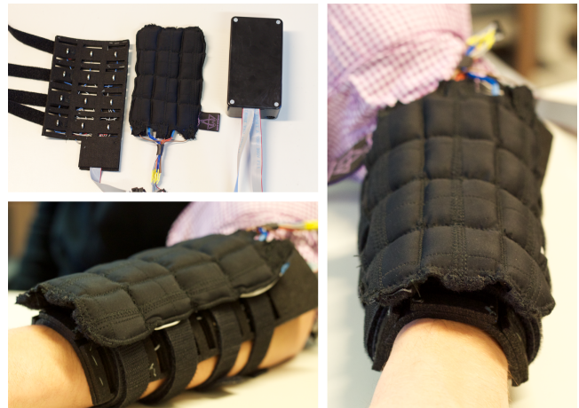
Figure 4: TaSST 1.5. In the top-left the output layer, input layer and control box can be seen.
